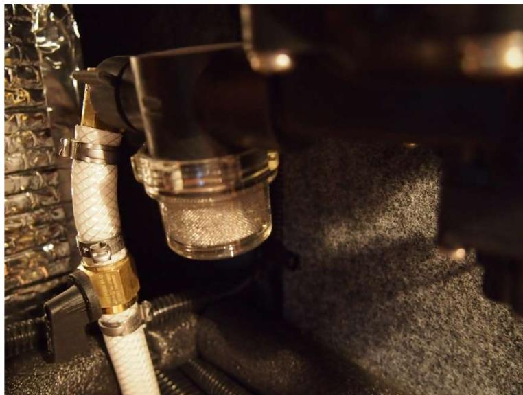
4. If you want the anti-freeze drained from the toilet cassette flush tank, all you need to do is pull the water level tube (located on the exterior portion of the toilet) from its upper fitting, and let the water/antifreeze drain out, and then put the hose back in place when finished. Note: it isn't necessary to drain the antifreeze in the flush tank if one doesn't desire to do so.
