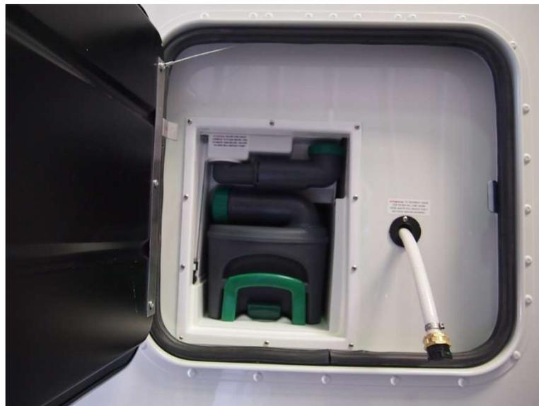
If your sleeper is equipped with a secondary fresh water tank, your fill system will typically appear as shown below.
