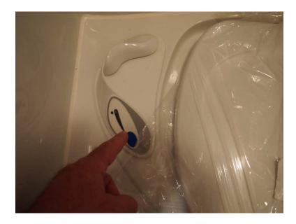
The toilet comes with chemicals that can be poured into the cassette unit from <u>outside</u>. <u>**Do not**</u> add the chemicals from inside the toilet to the flush water, as they will damage the seals in the toilet. Always add chemicals to the cassette on the outside of the unit.
