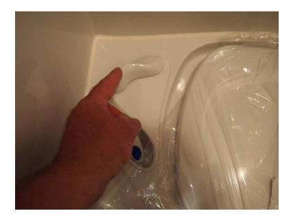
This button, shown below, is used to fill the toilet bowl with clean flush water.
