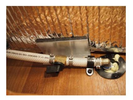
To fill the water tank, connect a fresh water hose to the water fill hose located on the exterior of your truck. You will know that your water tank is full when you hear or see water from the overflow valve running out on the ground. Then, simply turn on your water pump located on the systems control panel inside your sleeper. You're now ready to use your water system.
